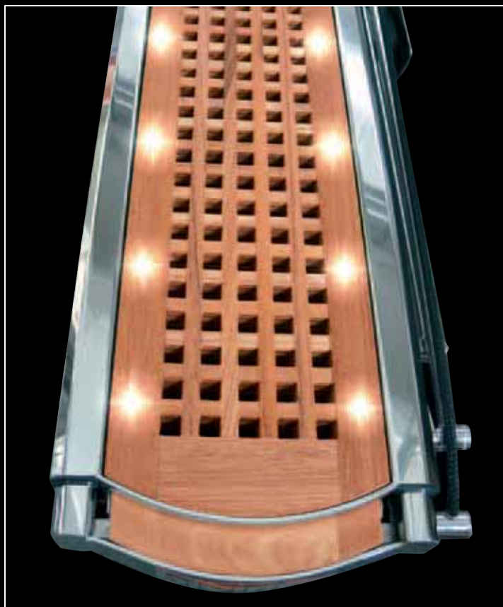
Illuminazione a led / Led lighting system
